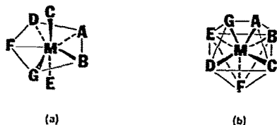
Fig. 7. Bimolecular or associative intermediates for octahedral substitution reactions; (a) pentagonal bipyramid of pseudo D_{5h} symmetry; (b) octahedral wedge of pseudo C_{2v} symmetry.
